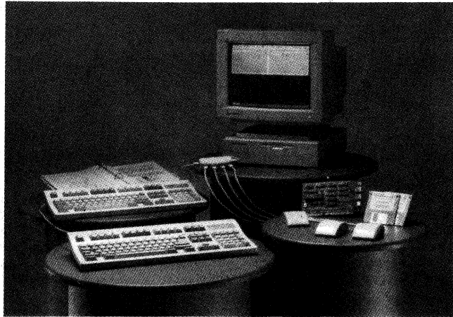
ACCESS.bus is a serial bus that supports "hot" attachment of up to 125 devices to a PC via a daisy-chained type of connection. Each device has its own address and is "recognized" by the system.
